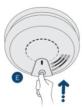
AFTER THE BATTERY IS INSERTED, WAIT AT LEAST FOR 3 MIN.AND ONLY THEN PRESS AND HOLD THE TEST BUTTON FOR **2 SEC.**
