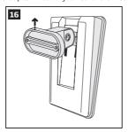
ATTENTION: Ensure that the holder is properly fixed into the device, otherwise it will prevent from using the back tamper switch for supervision of the enclosure's back side. If you do not wish to use the back tamper switch still, please disable it by setting a jumper on DIS-TAMP2 pins (see 2.2. Main Unit and LED Functionality).
